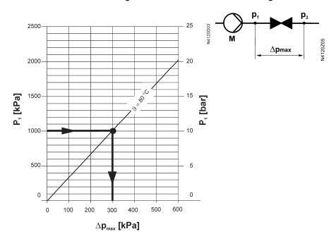
$\Delta p_{\text{max}}$  = Differential pressure with valve almost closed, at which cavitation can largely be avoided
