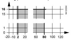
Working pressure and medium temperature as per ISO 7005 Current local legislation must be observed.
