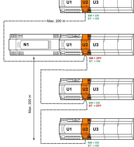
Decentralized subisland without power supply module (maximum distance depends on current on conductors CS and  $\perp$ )
