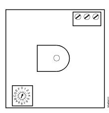
Address switch inside the housing.
