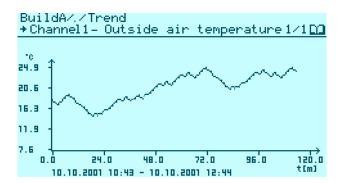
The PXM20-E operator unit provides the user with five channels for trend logging, enabling 5 data points to be logged.
