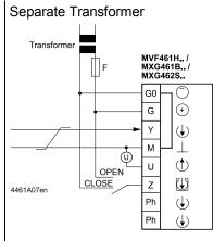
Terminal assignment for controller with 3-wire connection
