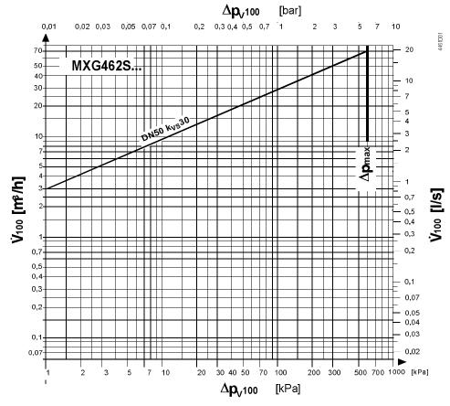
$\Delta p_{v100}$  = differential pressure across the fully open valve and the valve's control path by a volumetric
